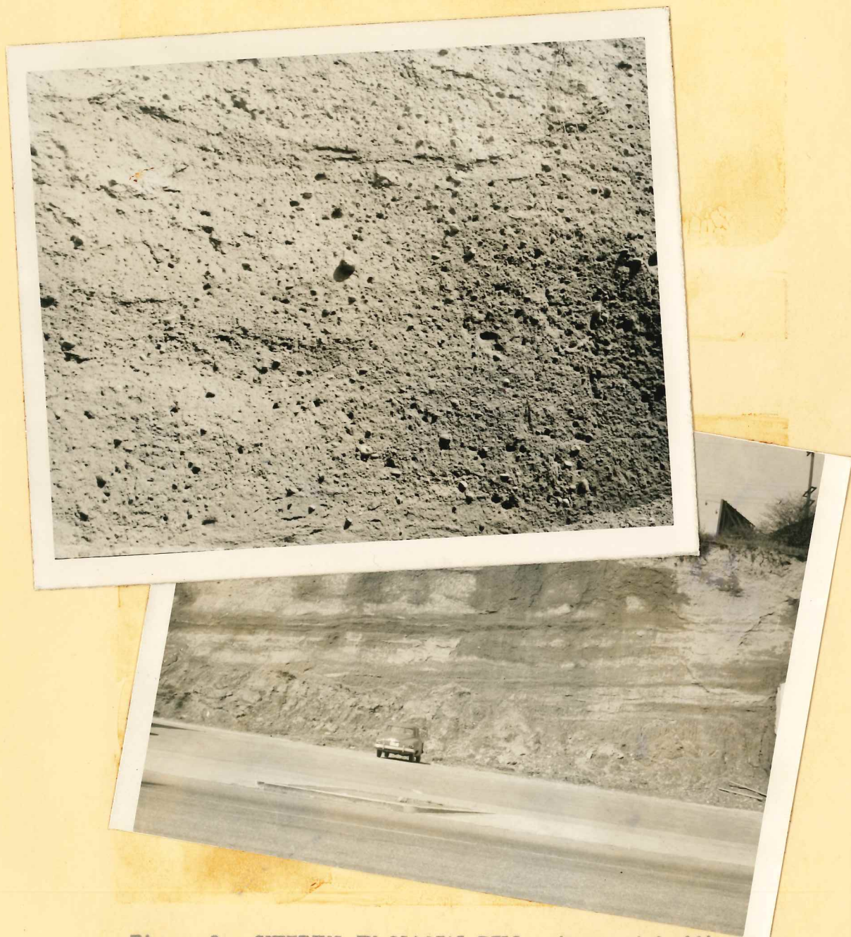
Figure 9. SHEETING IN GLACIAL TILL. Apparent bedding in photograph is structure due to ice movement.
