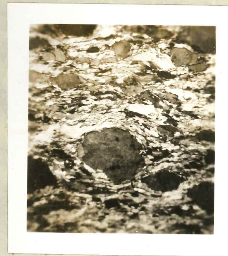
Feldspar-porphyroblast quartzite mylonite from the Secret Creek gorge area (B 36b).
