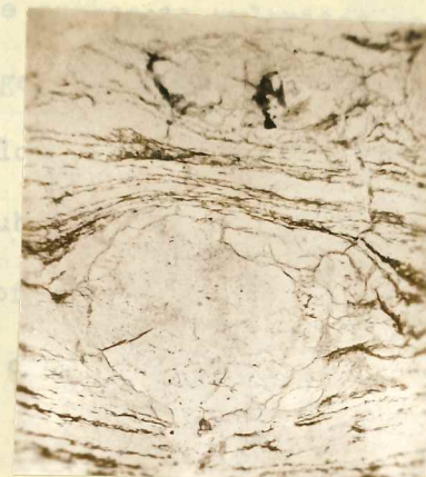
Fig. 29. Feldspar-bearing quartzitic mylonite. Note highly shredded biotite along wavy shear planes, the prominent feldspar porphyroclasts, and the thin layers of sheared quartz. Spec. B 40 (20 X magnification)
