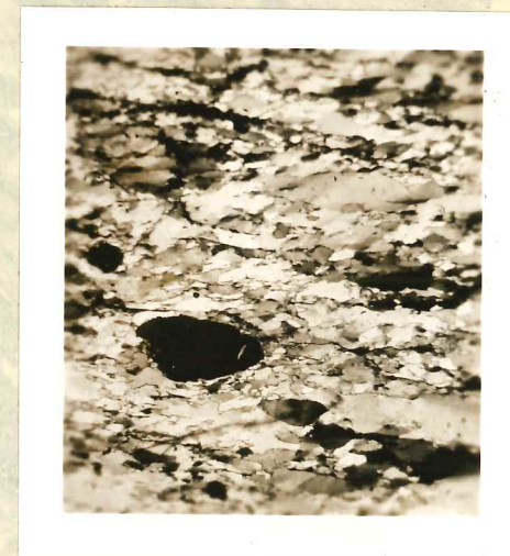
Feldspar-bearing quartzite mylonite (B 35). Feldspar grains occupied the now-void black spots in the photograph.
