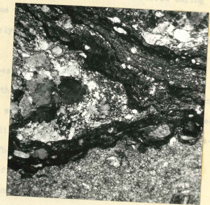
Fig. 44. Photomicrographs (plane light and crossed nicols) of impure carbonate mylonite in the Angel Lake unit near the Horse Creek thrust plane. Very fine-grained calcite is seen in the lower one-fourth of the photos. A portion of a large pod of a highly cataclastic quartz-feldspar-hornblende rock is seen in the upper three-fourths of the photos. Specimen B 85 ( 57 X magnification).
