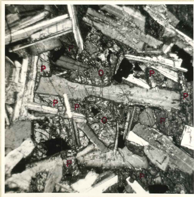
Fig. 9. Ophitic-textured diabase from middle conduit. 0 = olivine, P = clinopyroxene. (57 X magnification, crossed nicols).
