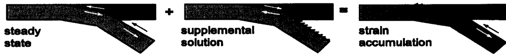
Figure 3.2. Elastic dislocation model of strain accumulation for a subduction zone. Arrows are the directions of plate movement. Streak lines indicate the locked place. (Savage 1983)
