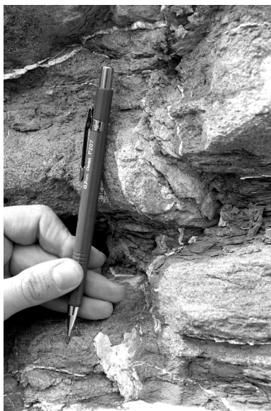
Figure 3.14. Photograph of a complex vein from the damage zone of fault BC1. The vein shows evidence for episodic dilation and cementation; deposits from ten distinct cementation events can be observed macroscopically.
