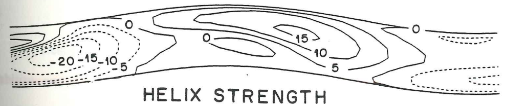
Figure 3.19. Predicted flow variables for run S-25 at equilibrium conditions. Contours intervals for topography, normalized bottom stress, normalized sediment flux, and helix strength are 0.2 cm, 0.1, 0.2, and 5^\circ , respectively.
