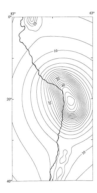
Figure 14. The plate geoidal anomaly for 80 km thickness and 350 km extension with a 1 m contour interval. The plate density is the same as for figure 12.
