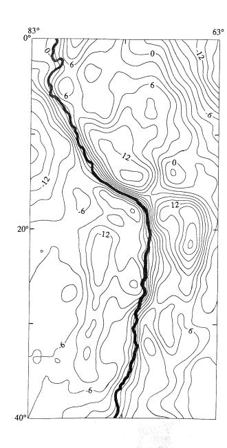
Figure 20. The complete (trench, plate sections) trial and error geoid for  $350 \, km$  extension and  $50 \, km$  plate thickness, contoured at  $2 \, m$  intervals. Adjusted parameters appear in the third column (second position) of table 3.
