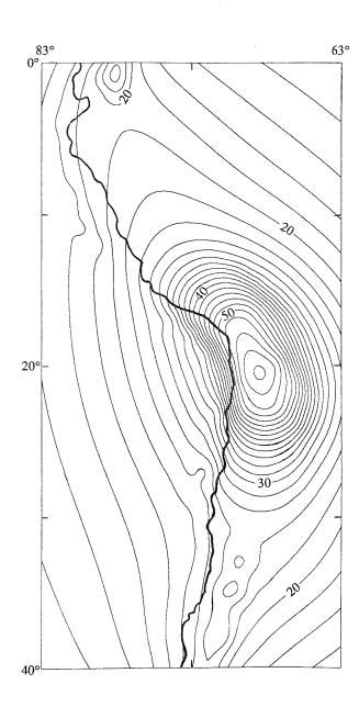
Figure 12. The plate geoidal anomaly for 50 km thickness and 350 km extension as for figure 11. Contour interval is 1 m.
