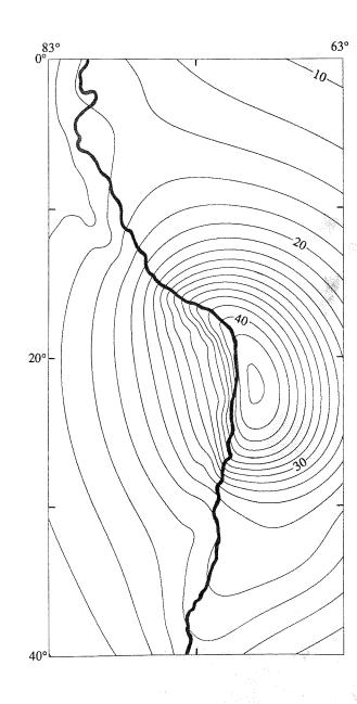
Figure 19. Least square section residuals for 50 km plate thickness and 350 km extension as for figure 18. The contour interval is 2 m.
