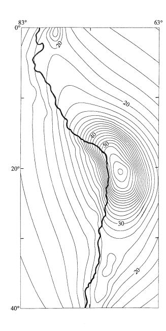
Figure 16. The complete (trench, plate, topography) least square geoid for 350 km extension and 50 km plate thickness, contoured at 2 m intervals. Corresponding parameters appear in the last row of table 1.
