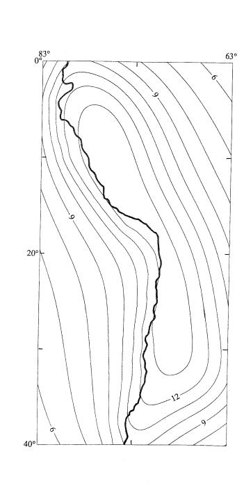
Figure 15. The complete (trench, plate, topography) calculated geoid for the 250 km extension and plate thickness of 50 km, contoured at 2 m intervals. Adjusted parameters are listed in the third row of table 1.
