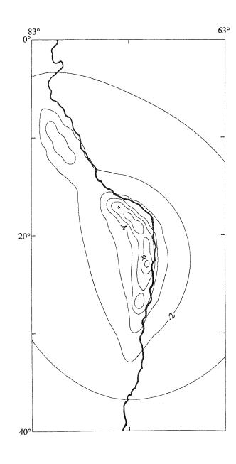
Figure 11. The complete (trench, plate, topography) calculated geoid for the 350 km extension (described in text) and plate thickness of 50 km, contoured at 2 m intervals. The corresponding adjusted parameters are listed in the second row of table 1.
