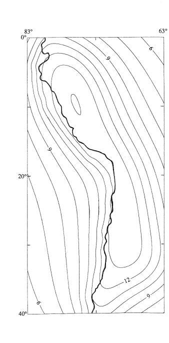
Figure 13. The geoid anomaly due to major continental topography, modeled by volcanism corresponding to the 350 km extension (best-fit with 50 km thick plate) as for figure 11. The contour interval is 2 m.
