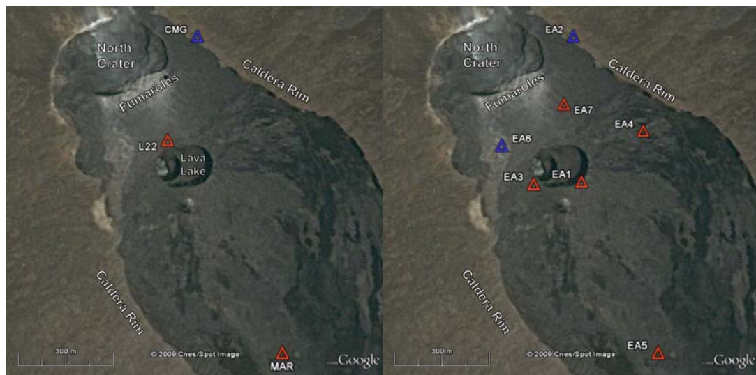
Figure 2.3. Station maps of temporary seismometers from each Erta 'Ale experiment, superimposed on aerial photographs. Notable features of the Erta 'Ale summit caldera are indicated. Short-period sensors (L22 and LE3D) are indicated by red triangles. Broadband sensors (CMG-40T) are indicated by blue triangles a. Seismometers of the Feb 2002 experiment. Position of lava lake is consistent with that of the photograph, just left of indicative text (see Fig. 2.2a). b. Seismometers of the 2003 experiment. The lava lake was smaller than suggested in the underlying aerial photograph, occupying only the center of the deeper pit region, NNE of station EA3 (see Fig. 2.2b). Lava lake label has been omitted to show detail.
