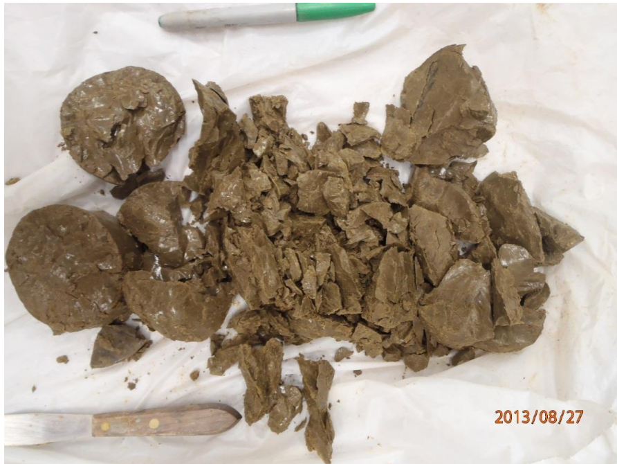
Figure 22: The contents of the Shelby tube taken at a depth of between 24 feet and 26 feet from borehole H-101vwp-13. I observed as I picked apart the silty clay the material could be easily separated by hand along abundant polished surfaces, especially in material from a depth of around 25 feet. Small metal spatula and Sharpie marker for scale.
