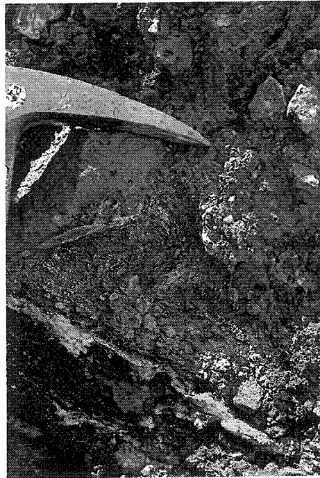
Figure 3.6. Scaly clay gouge. (a) arrows indicate a cross-section of a fracture in the hanging wall of the Copper Canyon detachment filled with scaly clay gouge (left) and a sharp slip plane that cuts large clasts of basalt and carbonate (right). (b) Scaly clay gouge filling a fracture above the Badwater detachment. The fracture is near a fault in the hanging-wall sediment (not shown).
