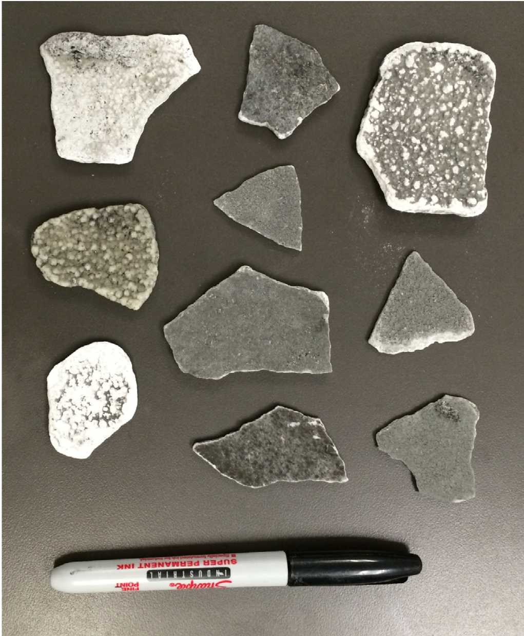
Figure 6. Scale chips collected from filter screen in place to prevent large material from entering Ormat power generators. Chips were chosen at random. Pieces exhibiting more rounding have likely been trapped in the screen longer than those with sharper edges.
