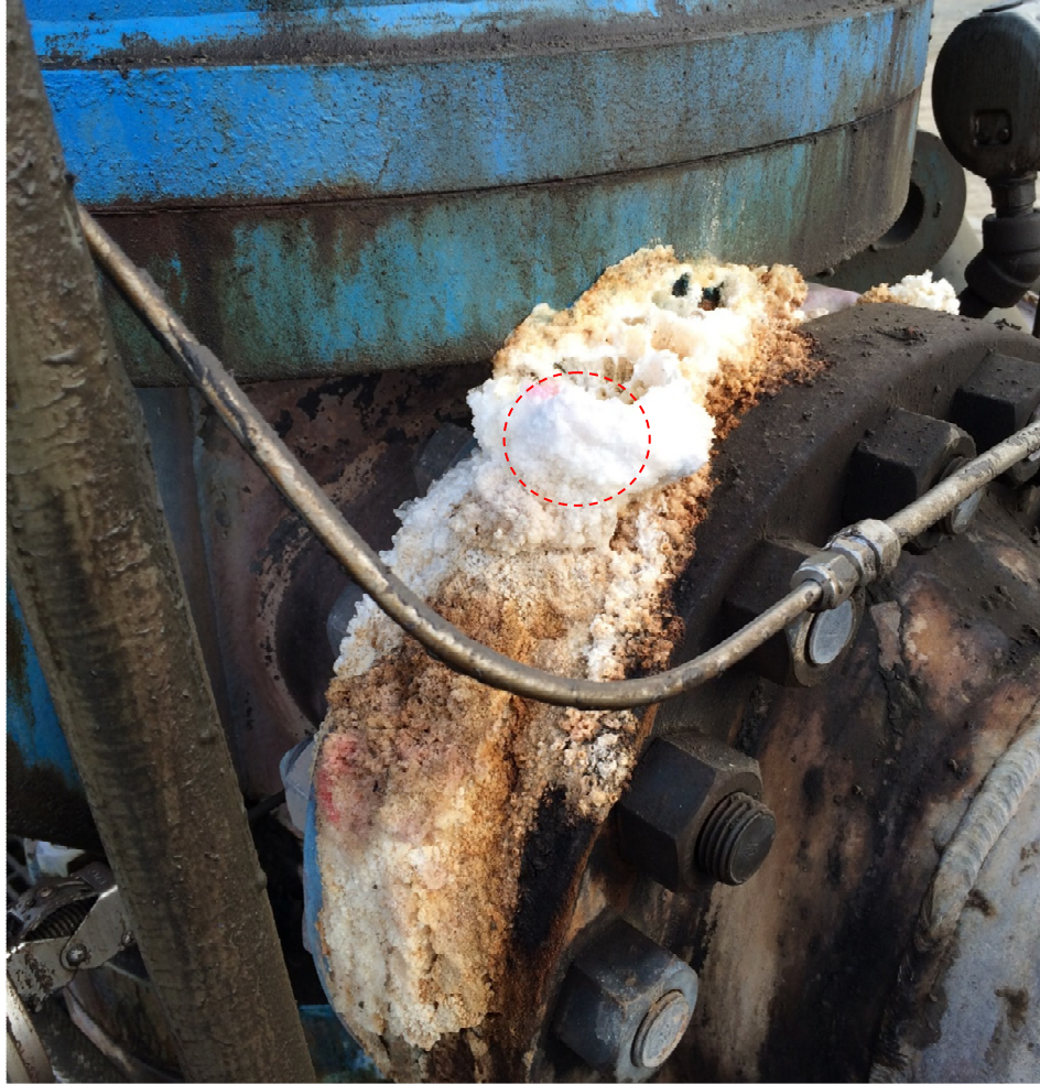
Figure 7. Material that has precipitated around a leak in the pump housing at production well 14-14. The red dashed circle indicates the approximate location where sample calcite sample 14-14 was collected. The source/cause of the staining is unknown; however, one possibility is the oil used to lubricate the pump shaft. The amount of CO 2 released during phosphoric acid digest indicates that it is 0.25% pure carbonate.
