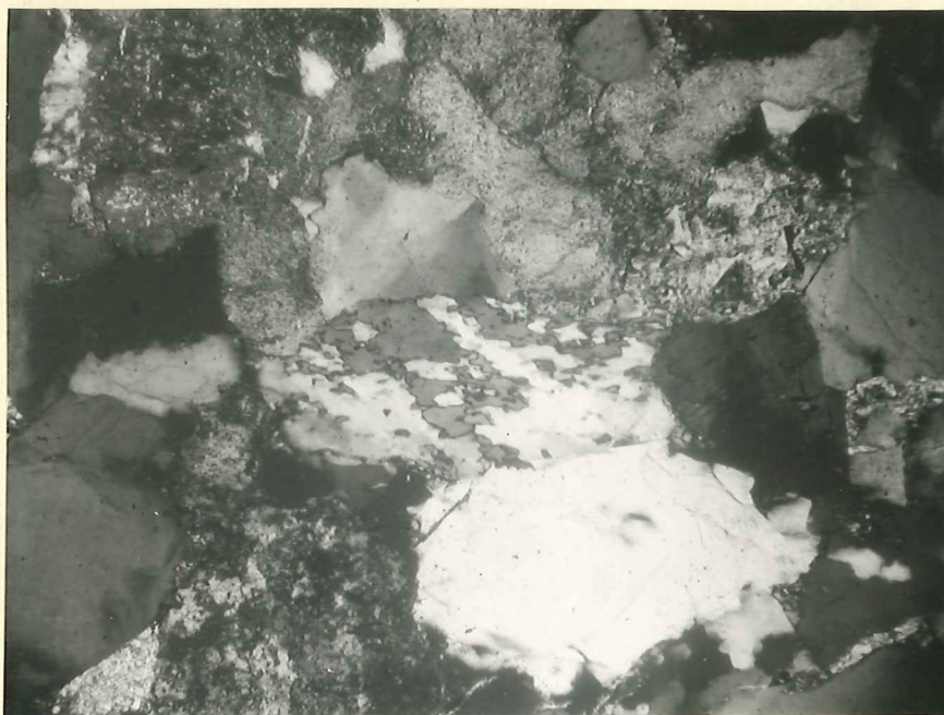
Specimen 17: Arkose, Puget Group. Pavement-textured quartz pebble and strained quartz grain. X 400, crossed nicols.
