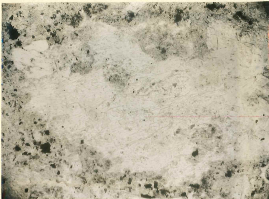
Figure 1. Specimen 34: Laharic Breccia, Keechelus Group. Authigenic plagioclase with highly irregular borders. X320, plain light.
