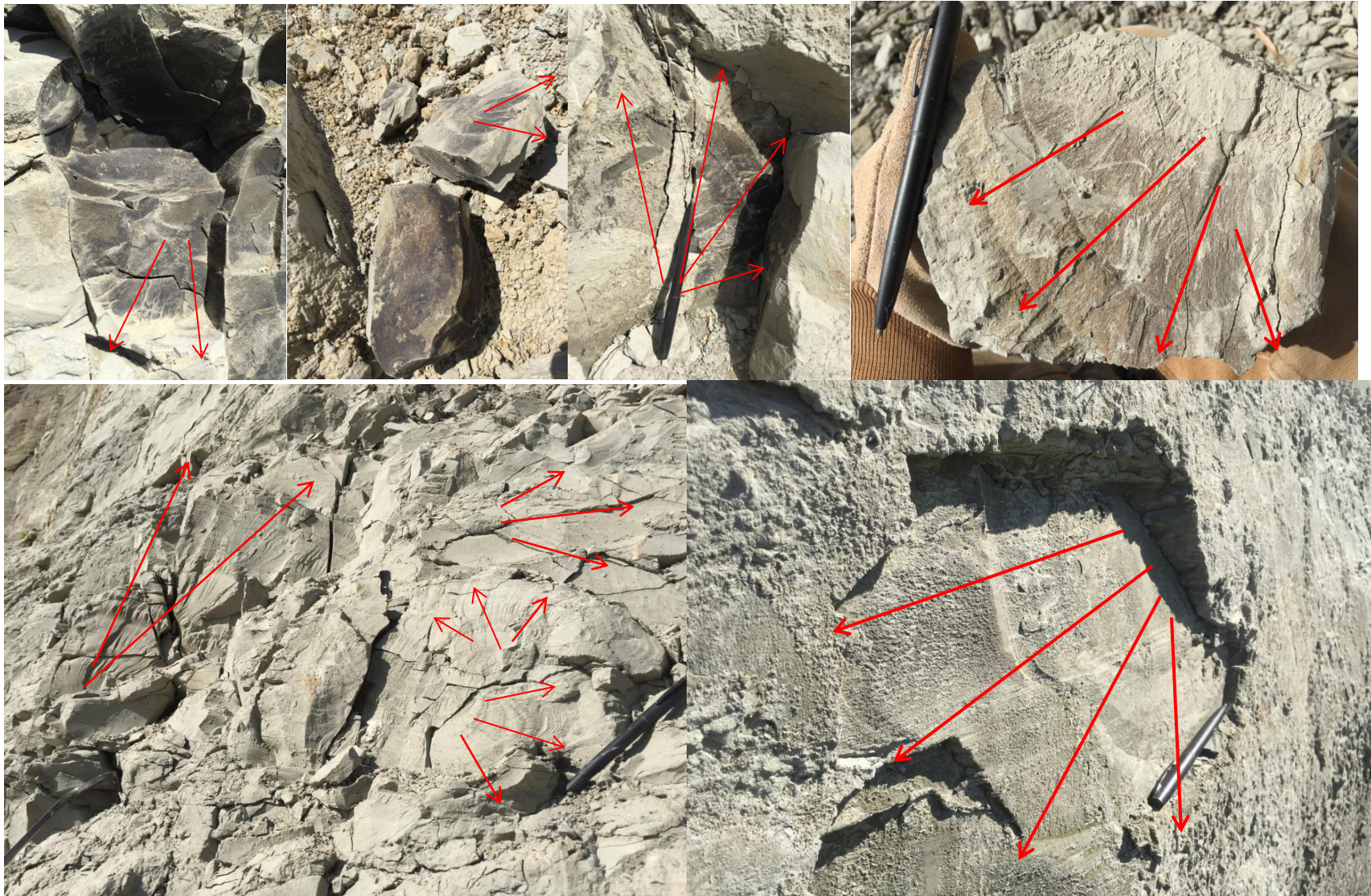
Figure 16: Radial plumose surface texture and concentric arrest marks in the clay, marked with red arrows that indicate the directions of fracture development out from a (or several) point(s) of origin.
