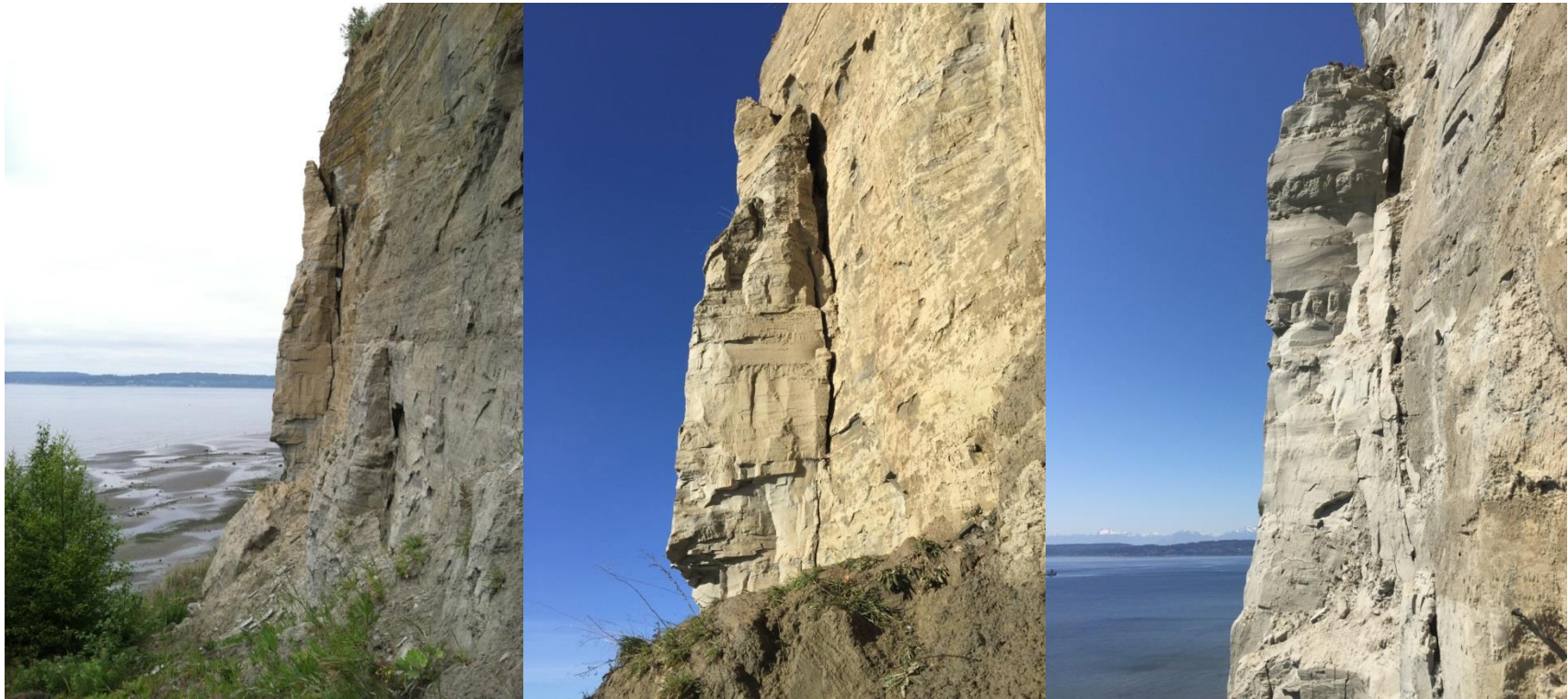
Figure 9: Photos taken 5/17/2015, 11/21/2015, and 4/20/2016 respectively showing the change occurring over time at a distinctive fractured wedge at the northwestern corner of the bluff.
