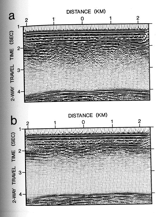
Figure 17. a. Lower migration velocity version of Line 4B after running stack. O distance is center of axial valley. Arrow on lower border shows location of the shot used for the spectrum in Figure 18a. b. Higher migration velocity version of Line 4B after running stack. O distance at center of axial valley. Arrow on bottom border shows location of shot used for the spectrum in Figure 18c.
