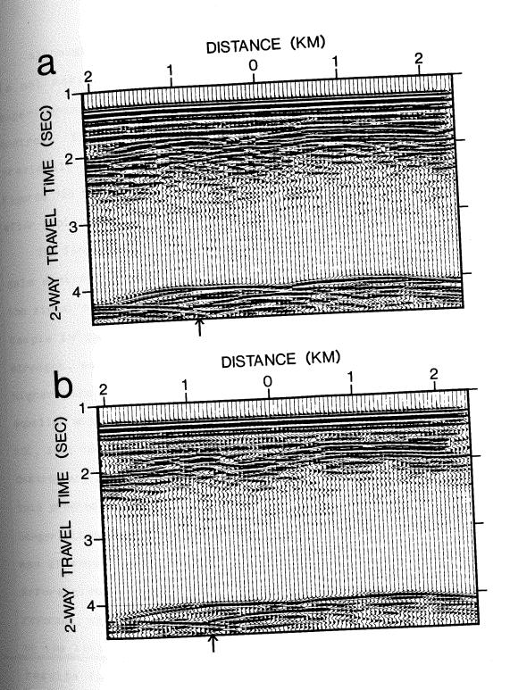
Although the need for an additional stage of band pass filtering is not obvious from an examination of Figures 17a and 17b, experimentation showed it to improve the results of automatic gain control. The same band pass filter was used as had been applied previously. Representative line spectra of the data can be seen in Figures 18a - 18d. Figures 19a and 19b show the data for Line 4B after application of the filter.
