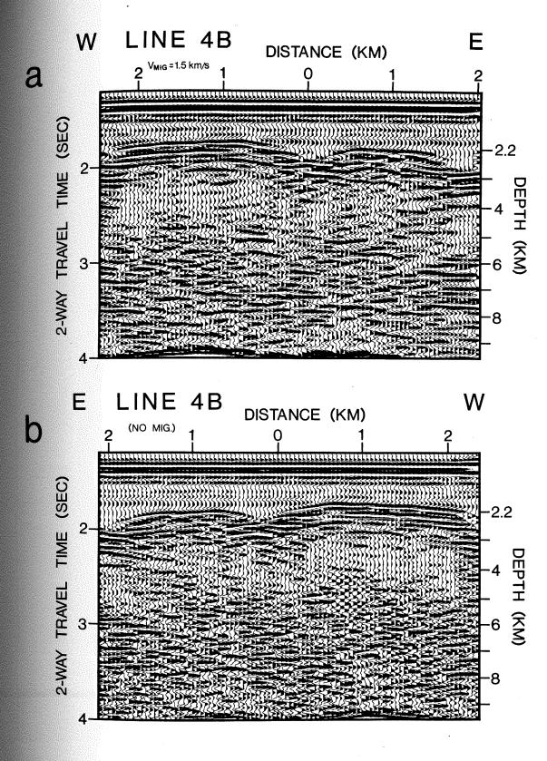
Final processed version of Line 4B. The higher mid-crustal migration velocity has been used. This profile has been reversed so that E is on the right; O distance is at the center of the axial valley. Figure 21.
