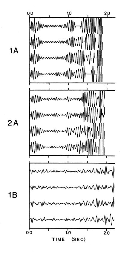
Figure 28. Results of the gain test for Lines 3B, 4B, and 8A. On many of the traces there is a jump in amplitudes at roughly 1 second, relative to the background exponential increase.
