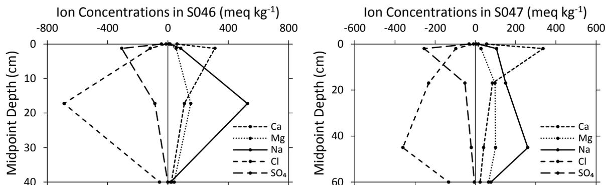
Figure 2.8. Graph showing the depth distribution of major anions and cations in two soils from Bonney Basin. Soil S046 is located at 86 m elevation, and soil S047 is located at 116 m elevation. Ion distributions indicate that significant leaching of Cl salts has occurred following evapoconcentration of salts near the soil surface.
