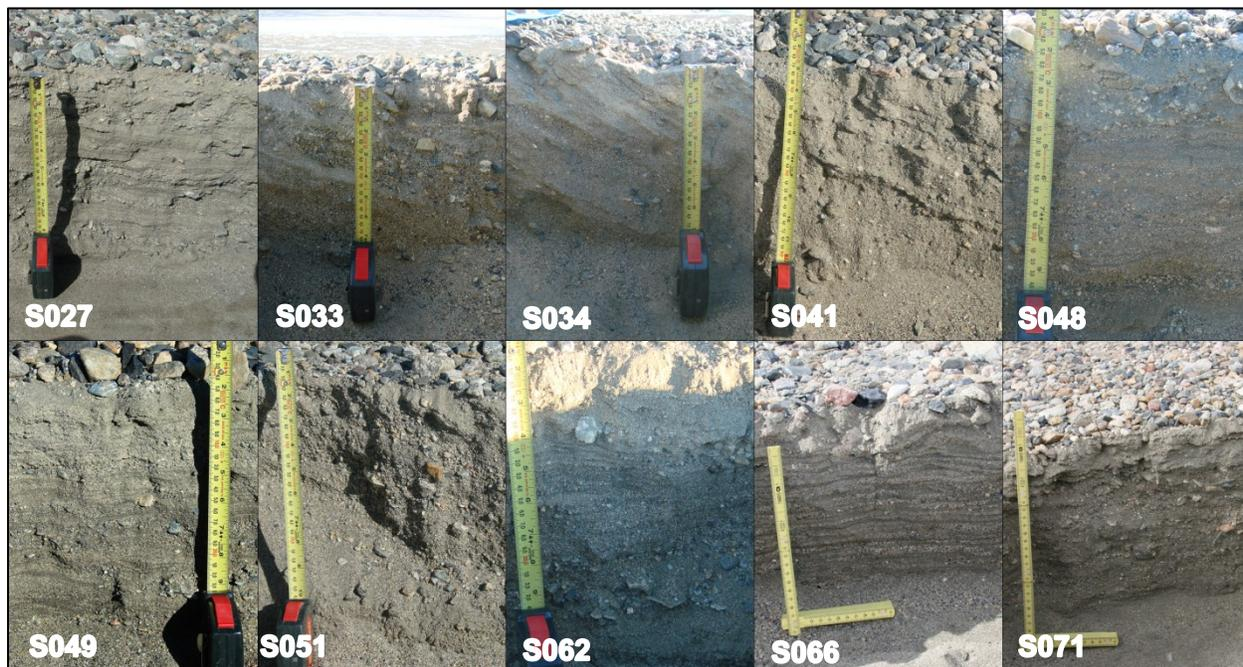
Figure 4.3. Soil profiles in terraces sampled for luminescence dating. All soils are composed of medium to coarse-grained sand and have either cross-bedded or foreset fluvial stratification.
