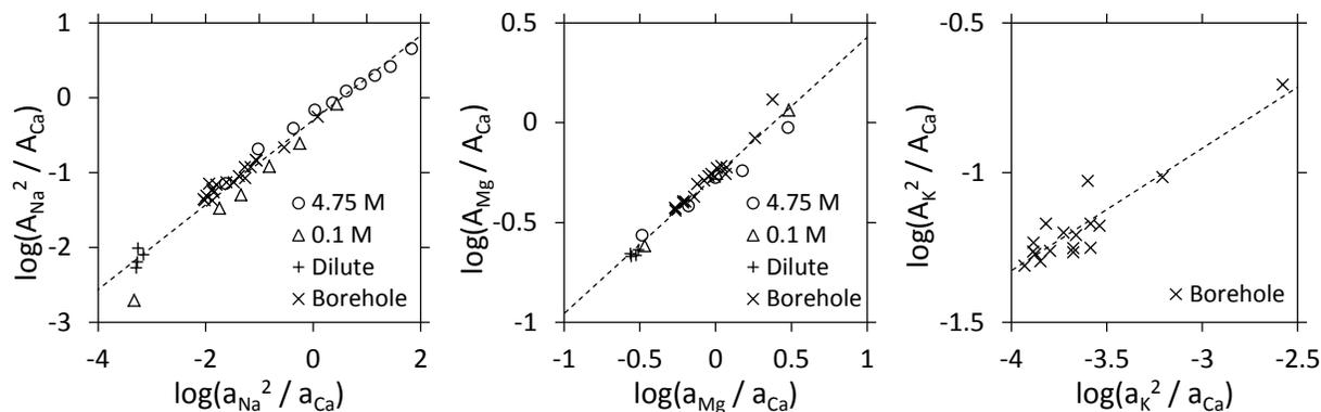
Figure 3.7. Plots of  $\log(A_j^{z_i}/A_i^{z_j})$  versus  $\log(a_j^{z_i}/a_i^{z_j})$  for Ca-Mg, Ca-Na, and Ca-K exchange for all exchange experiments. The dashed lines are a linear fit to the experimental data, with the Rothmund-Kornfeld parameter  $n^{ij}$  obtained from the slope and  $\log K^{ij}$  from the intercept.
