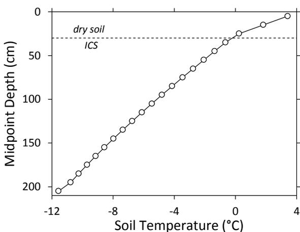
Figure 3.10. Average temperature profile for the Taylor Valley borehole when the soil surface is above 0°C modeled using equation (11) and soil temperature data from the Lake Fryxell LTER met station. The depth to ice-cement is indicated by the dashed line at 30 cm depth.
