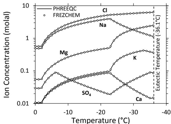
Figure 3.2. A Graph showing seawater freezing modeled with PHREEQC and FREZCHEM. The initial composition of seawater was: Ca = 0.01074, Mg = 0.05474, Na = 0.48610, K = 0.01058, Cl = 0.56672,  $\text{SO}_4$  = 0.02927, and  $\text{HCO}_3^-$  = 0.00238 molal in equilibrium with atmospheric  $\text{CO}_2$ . Although not shown, pH and inorganic carbon species calculated with the updated PHREEQC are also in excellent agreement with FREZCHEM.
