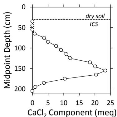
Figure 3.8. A graph of the CaCl<sub>2</sub> component in the borehole, defined as the equivalent concentration of Ca in excess of HCO<sub>3</sub> and SO<sub>4</sub> ( $\text{CaCl}_2 = 2\text{Ca} - \text{HCO}_3 - 2\text{SO}_4$ ). The depth to ice-cement is indicated by the dashed line at 30 cm depth.
