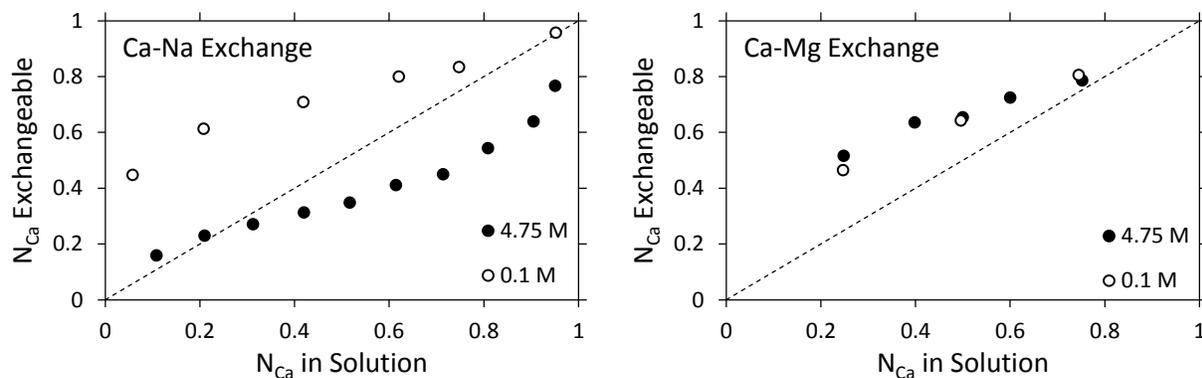
Figure 3.6. Cation exchange isotherms derived using data in Table 3.2 and Table 3.3 for 0.1 M and 4.75 M solutions.  $N_{Ca}$  is the equivalent fraction of Ca in either the solution or exchange phase. The dashed line is the isotherm for which cations are equally partitioned between exchange and aqueous phases.
