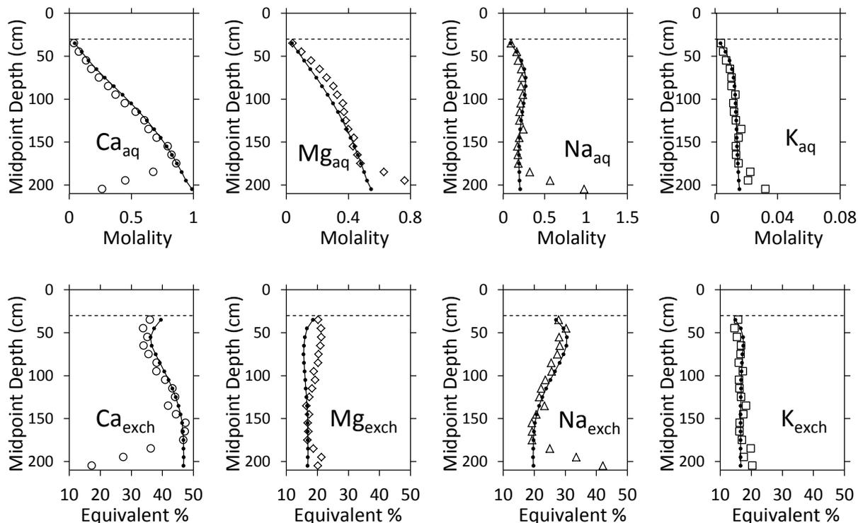
Figure 3.13. Graphs showing the distribution of aqueous (aq) and exchangeable (exch) cations predicted from the transport model compared to the modeled frozen state of the borehole. Black points connected by lines indicate values from the transport model, while white data points are values from modeling freezing of the borehole in Figure 3.11. The depth to ice-cement is indicated by the dashed line at 30 cm depth.
