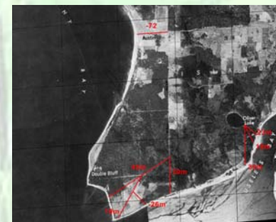
Fig. 5: Quantitative assessment of shoreline retreat can be determined by measuring difference in shoreline positions on the two images with known geo-referenced structures that have been present over past 60 years. Note that the erosion values given here are not adjusted to account for the angle of incidence between the transect line and the shoreline. Only those transect lines that intersect the shoreline perpendicularly will provide accurate estimates of the erosion magnitude.
