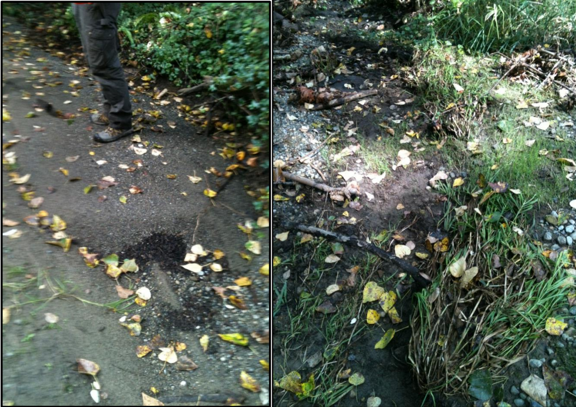
Figure 24. Photograph of a fresh deposit of fine sediment after heavy rains (left) and blown vegetation in the direction of flow (right) within the study-reach.
