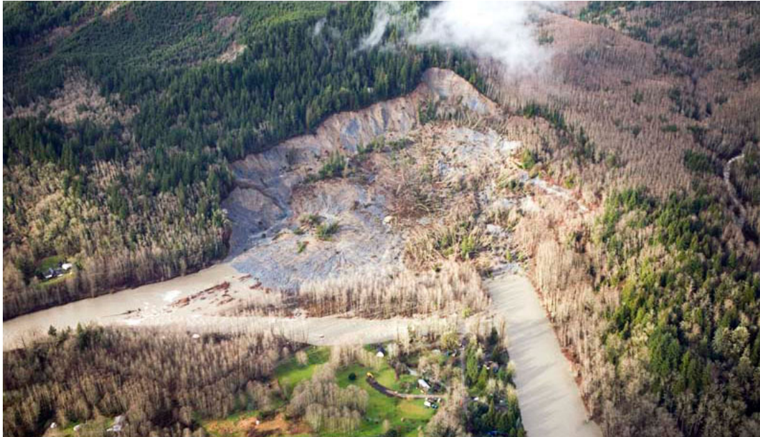
Figure 4.3A: Field example of a fine-grained landslide dam on the N.F. Stillaguamish River. Flow is from right to left in the photograph. Aerial photos dating back to 1933 and the 1890 land survey maps show reactivation of an ancient landslide by chronic bank erosion at the outside meander bend. Reactivation of the landslide delivers large pulses of glaciolacustrine sediment to the N.F. Stillaguamish River every 10 – 20 years. The most recent failure in January 2006 completely blocked the N.F. Stillaguamish River with fine sediment and woody debris. The emergency cutoff channel shown in the photo was excavated through the meander bend by the Army Corps of Engineers to alleviate flooding of riverside homes caused by the backwater impoundment. Photo credit: Dan Crowell.
