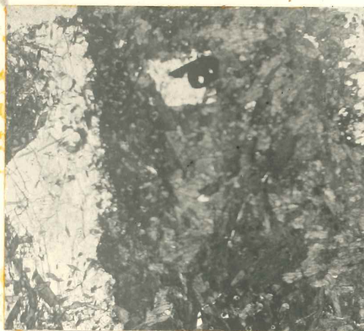
Figure 12 Uraninite veinlet in shear between orthoclase and hornblende. Pl. light. Loc. 13. Section M-4.
