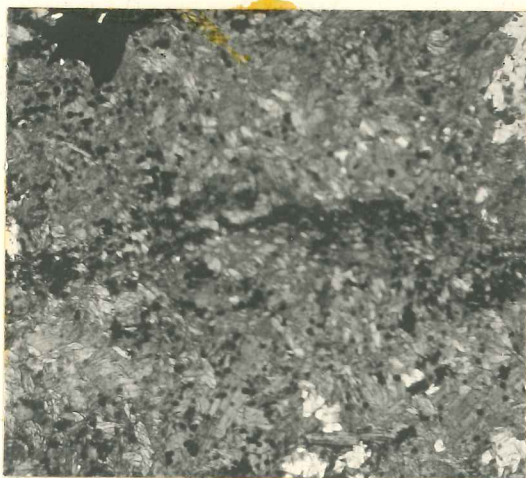
Figure 11 Uraninite in hornblende shear. Actual crystals are much smaller than black spots, which are pleochroic halos. X 16. Pl. light. Loc. 1. Section A-3.
