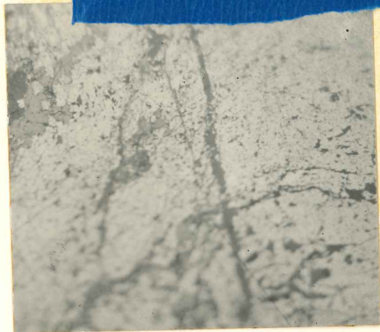
Figure 20 Uraninite and molybdenite veinlets in arsenopyrite. Uraninite (black) forms crystals along fractures in arsenopyrite. X 16. Polished sec. Loc. 2. Sec. E-1.
