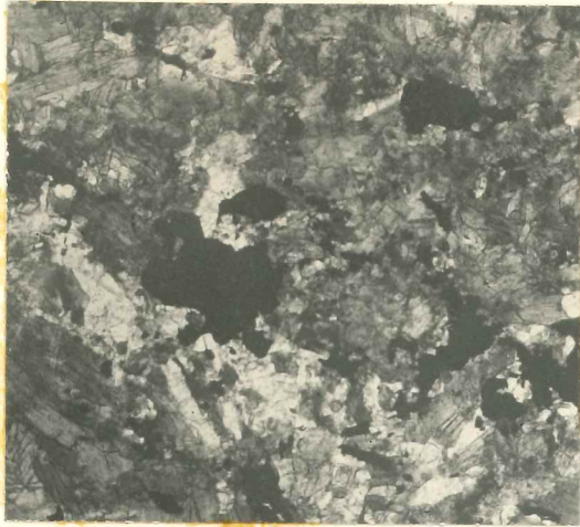
Figure 7 Molybdenite (large grains) and uraninite in hornblende and apatite. The Uraninite occurs as small grains in molybdenite and hornblende. X 16. Plain light. Loc. 12. Section C-10.
